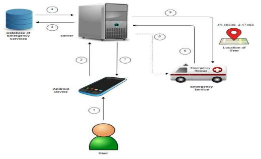
Figure 3-1: Flow Diagram of Case-1 (When the Nearest Service is Available)
